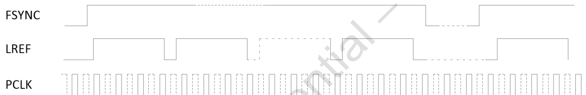
Figure 1-7 DVP timing diagram
